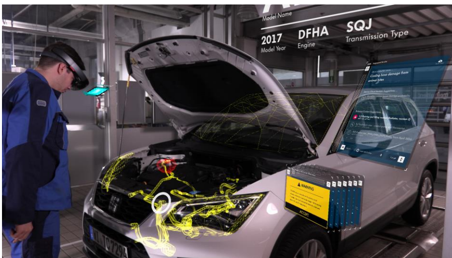
The on-screen display of additional parts information alongside animations depicting their assembly, accelerates the repair process.
